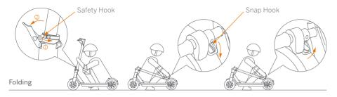
Turn off your KickScooter. Turn the safety hook counterclockwise and open the quick release lever.
