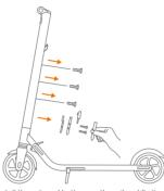
3. Install the external battery on the rail and fix it with the M4 (20mm) screws (2 pcs), provided with this product. After they are properly installed, block the screw holes with the rubber stopper.
