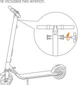
2. Firmly connect the wires inside the handle and the stem. Slide the handle onto the stem. Be aware of the correct orientation.
